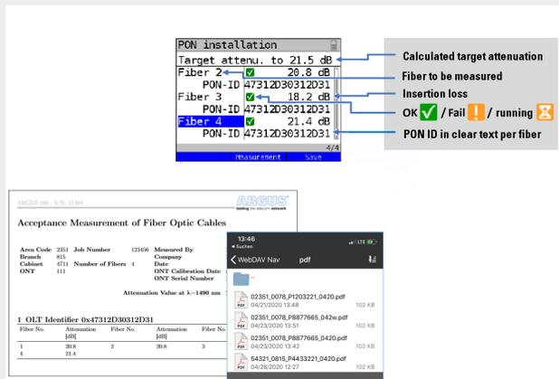
Figure 2: Example of a measuring wizard in an instrument (top) and an acceptance measurement log in PDF format on a PC (left) and a smart phone (bottom right).
