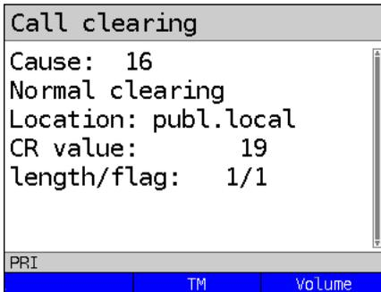
The ARGUS will display the cause (see the table below) of the disconnect (e.g. Normal clearing) and the location where the cause occurred (e.g. subscriber). Depending on the access, additional information will be displayed (in this example, Units).
