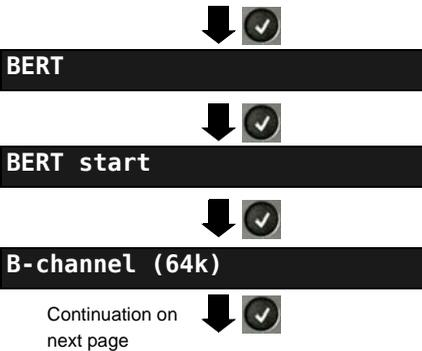
In the case of a PRI access in end-to-end mode (see page 129), a BERT can be run:
