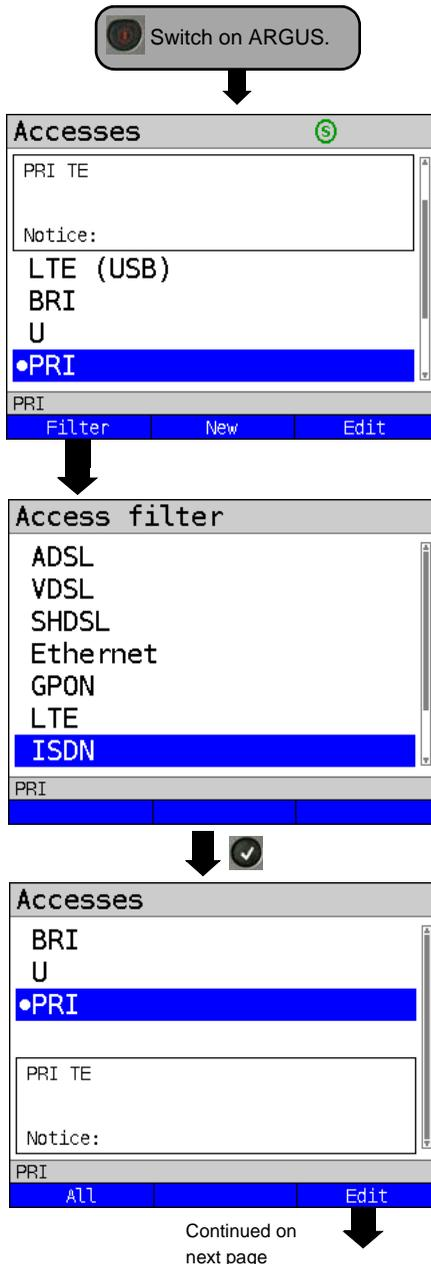
After powering up, ARGUS displays all configured accesses (up to 100). A default connection is configured for each access type.
