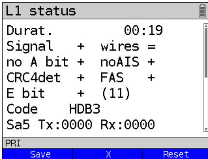
The ARGUS displays the time that has elapsed since the ARGUS was initially started or it was last reset in minutes and seconds (00:19).
