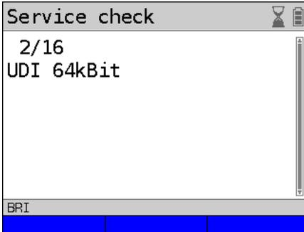
The ARGUS can resume an interrupted single test: In this example, the ARGUS is running a Service test.
