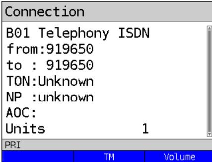
The connection is setup using B-channel 1.
