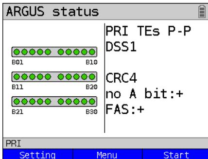
During this phase, the ARGUS displays the A bit of the remote side and the FAS. The protocol can only be determined when the A bit is not set (+). The FAS (Frame Alignment Signal) indicates whether the ARGUS could correctly synchronize with the incoming 2 Mbit data stream's alternating frame identification word or message word and the, perhaps present, CRC4-superframe structure.
