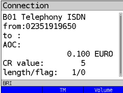
The connection is setup using B channel 1.
