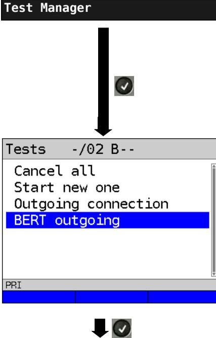
All tests will be terminated and all connections cleared down.
