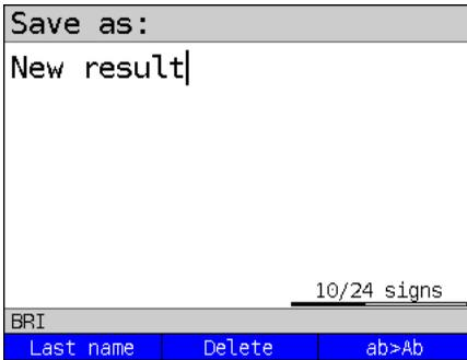
Select the memory location. For each memory location used, the ARGUS will display the name assigned to the memory location (in this example, New result).
